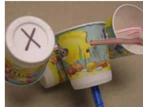
Your anemometer is ready to use! Count the number of times the X spins around. 10 spins per minute, or one spin every six seconds, is 1 mile/hour. How fast is the wind blowing?
