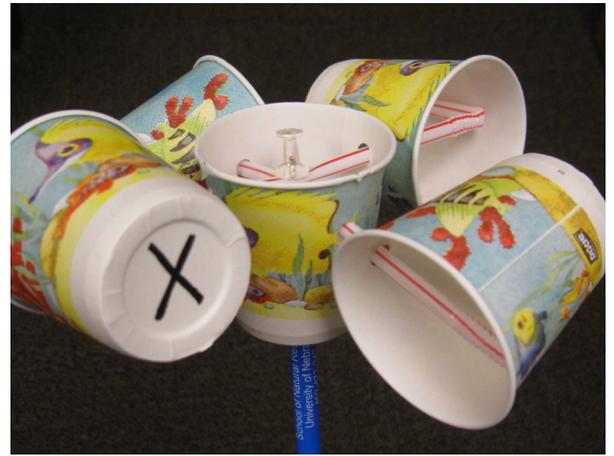
5) Push the other end of the straw through the five-hole cup and then through the hole in one of the one-hole cups. As before, tape the straw to the inside of the cup, making sure that the cups face opposite directions.
